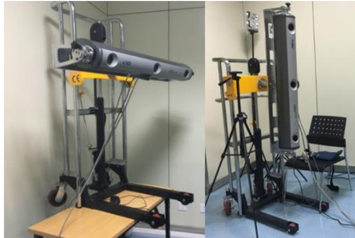
Figure 3. Position sensors of the motion capture system
